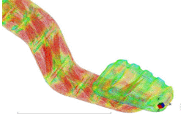
Figure 3. Fiber orientations predicted through Moldflow simulation.
